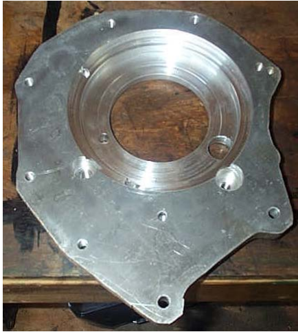
Figure 7 – 203 range box (front) side of adapter. Note multi-step profile of machining to accommodate bearing retainer basket. Also note two counterbored holes on bottom circumference of basket recess. These 2 counterbored holes contain bolts that retain the transfer case onto the rear of the adapter, but that thread from the front of the adapter.
