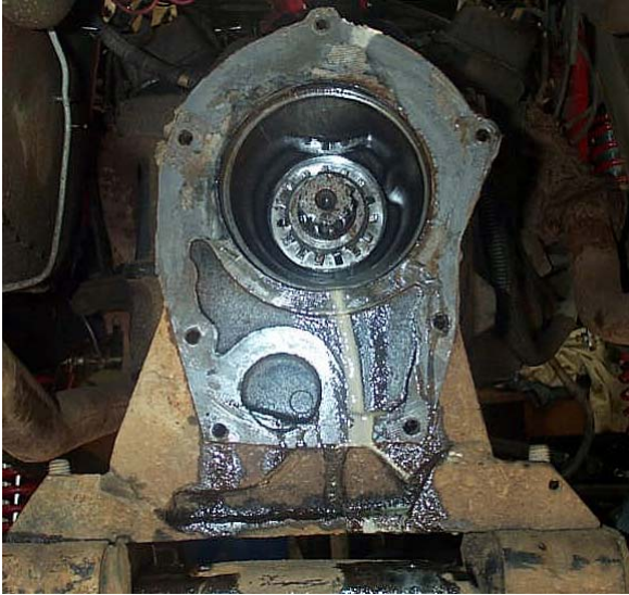
Figure 5 – Stock Chevy SM465 to NP203 adapter, showing asymmetrical 7-bolt pattern.
