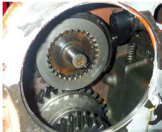
Figure 3 – large helical gears inside the 203 range box.
