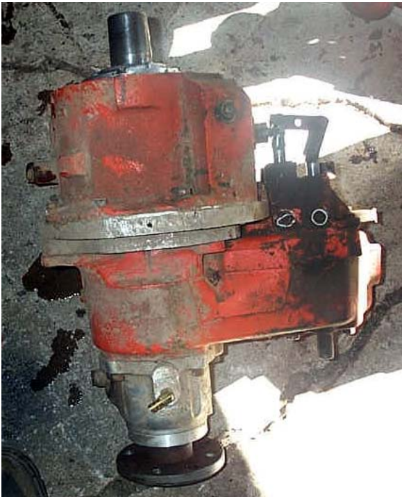
203 range box, adapter, and transfer case bolted together; ready for installation into the vehicle.
