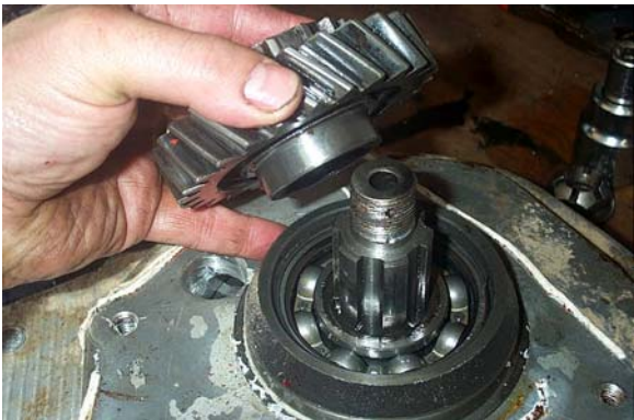
Transfer case input gear (main drive gear) being removed from Doublertm shaft.
