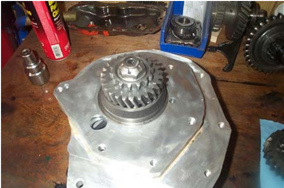
Transfer case input gear secured onto custom Doubler™ shaft with locknut using thread locking compound and torqued to 300 ft-lbs.
