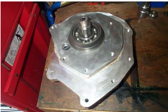
Bearing and retainer fit into recess machined into rear side of adapter.
