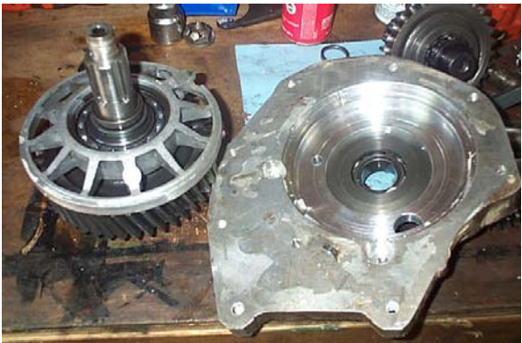
203 low-range gear with shaft, bearing, and bearing retainer "basket" removed from aluminum adapter.
