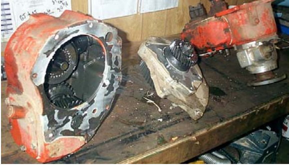
Disassembled components of the Doubler™, from left to right, 203 range box, adapter with shaft, Dana 20.
