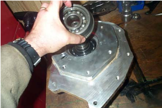
T150 3-speed transmission output bearing and retainer being placed over shaft on rear side of adapter.
