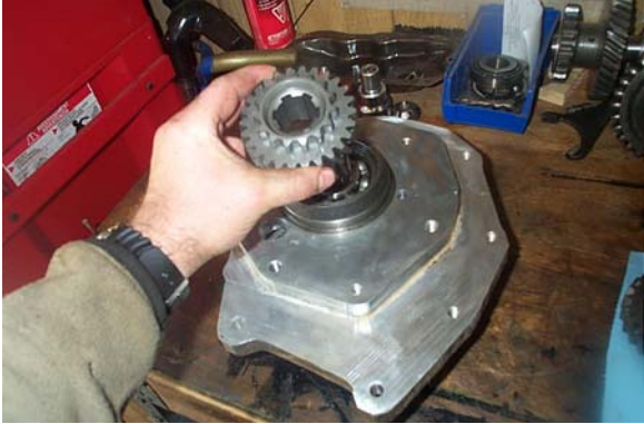
Transfer case input gear being installed on Doubler™ shaft.
