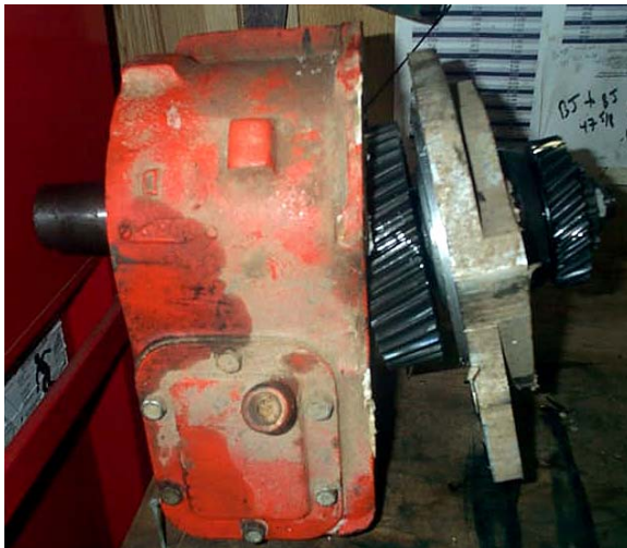
Adapter being removed from 203 range box. Note that the aluminum adapter is sandwiched between the 203 low-range gear and the Dana 20 input gear.
