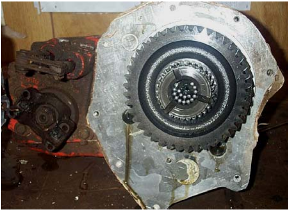
Adapter attached to transfer case. Note the two recessed bolts (just at the circumference of the large gear) that thread into the transfer case.
