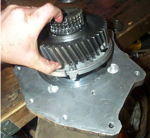
Shaft and gears being replaced in front side of adapter. Note locating tab on bearing retainer basket which fits into corresponding slot machined into adapter.
