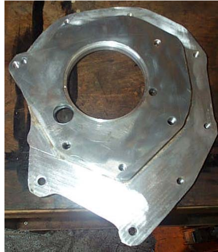
Figure 8 – Rear side of adapter, to which the transfer case mounts; machined to accept the T150 3 speed transmission output shaft bearing. Note the large hole that allows gear oil to flow from the 203 range box to the transfer case. This permits filling both cases with 85w gear oil from a single point on top of the 203 range box.
