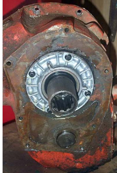
Figure 4 – Front input of Chevy NP203 showing asymmetrical 7-bolt pattern and 10-spline input indicating SM465 version.
