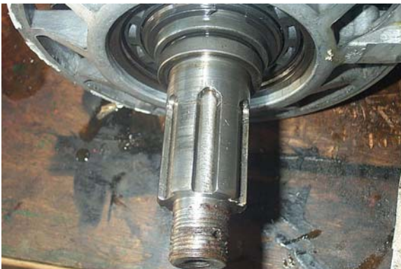
Figure 6 – Cut down and re-splined 203 output shaft.
